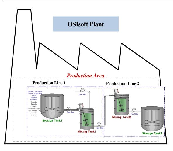
As shown here, each tank has different process variables such as Internal and External Temperatures, Flow Rate, Pressure and Level whose values are continuously collected from devices on the Plant. In the early days of PI System, these process variables were the only data items whose historical data could be stored in Data Archive.
